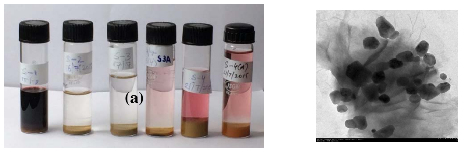
Figure: (a) Image of Synthesised Graphene oxide, (b) Transmission Electron Microscopy of synthesized Graphene Oxide.
